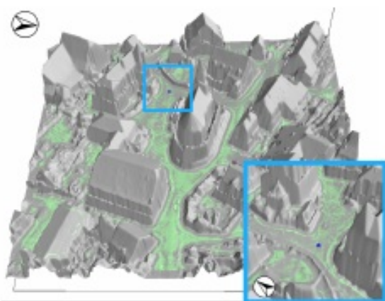
Fig. 6. Minimum traversability overlay of the Sullens map over 32 possible orientations. Blue square zooms in a region facing the central building.
